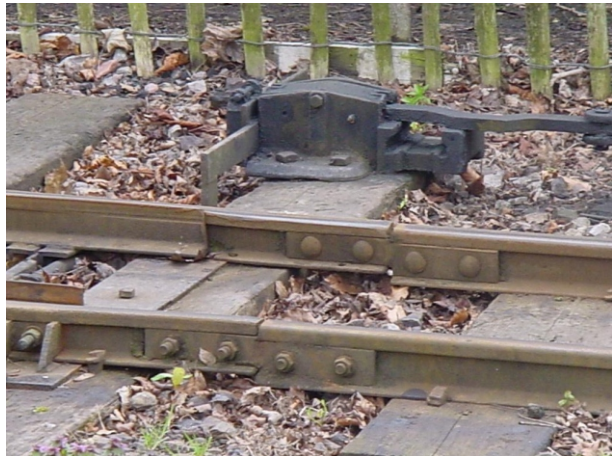
Figure 16. A bolt lock, on a narrow gauge railway (Leighton Buzzard) is usually placed in the centre of the "four foot" way - uses a more usual design of lock
