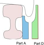
The table below explains what packing pieces (B or C) should do to the flangeway that is created by the simulation of tram track.
